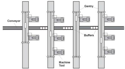
Fig. 1. Schematic of arrangement of structural components of RMS [14]
