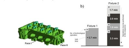
Fig. 2. Casing-class part to be manufactured in RMS: a) general schematic view of the product, b) structure of the product's technological process [16]
