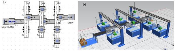
Fig. 4. Example of simulation model for configuration B developed using Tecnomatix Plant Simulation software: a – 2D model; b – 3D model
